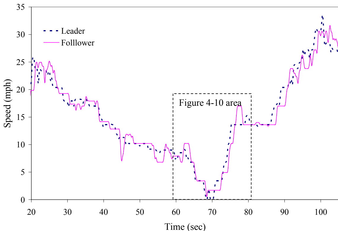
Figure 4-9. Field observed speed profiles of two following vehicles.
